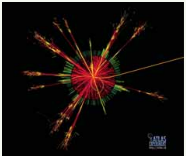
Fig. 2 Simulated interaction in the Atlas detector with all outgoing reaction products traversing the successive shells of the detector. The central region where most particles are colored red, represents the inner tracker detectors. The surrounding heavy calorimeters provoke showering around the absorbed particles. The yellow track to the right is an escaping muon. The scale of the figure is ~10m across. Photo CERN/Atlas.
