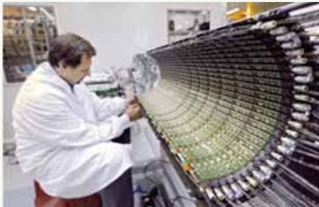
Fig. 7 Final assembly work on the Atlas pixel barrel (half). One can see the modules along the ladders. The white stubs are connecting tubes for the cooling channels, one for each ladder. Photo CERN/Atlas.
