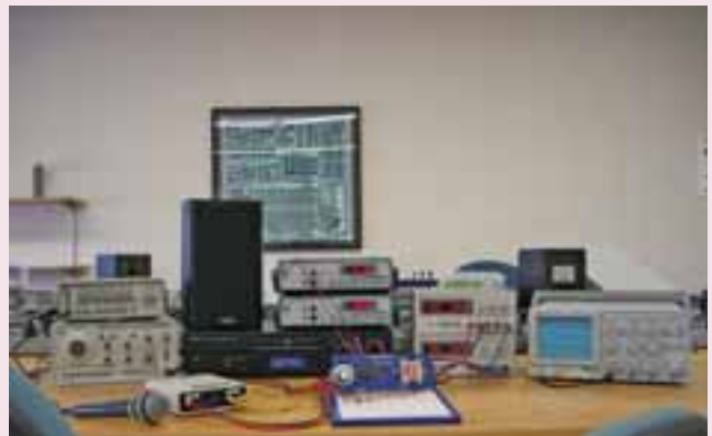
Fig. 1. Audio in the first circuits lab. A microphone, a CD/MP3 player, a small power amplifier, and a loudspeaker are standard equipment in each station.
