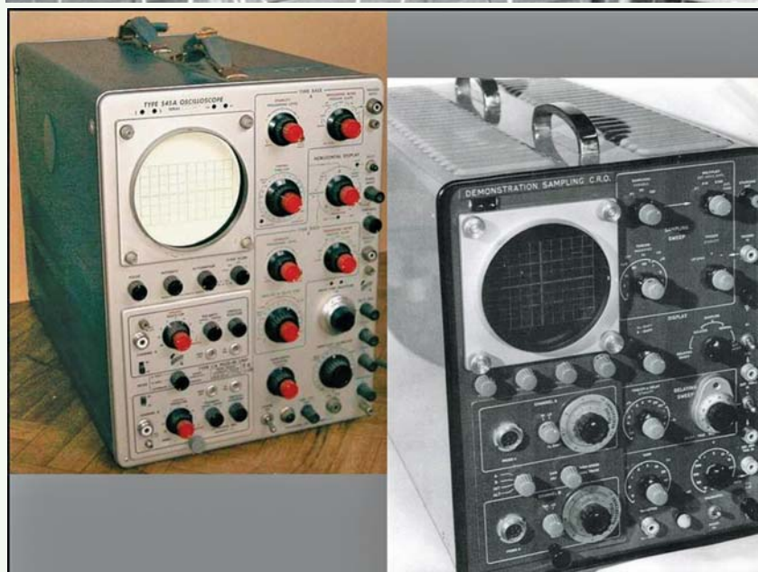
Figure 9: (a) The L362 oscilloscope (on the left) and my own sampling oscilloscope (on the right); a second plug-in can be seen. (b) Shows its similarity to the superb Tektronix 545 oscilloscope.
