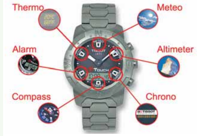
Fig. 7: Tactile areas on the Tissot T-Touch
