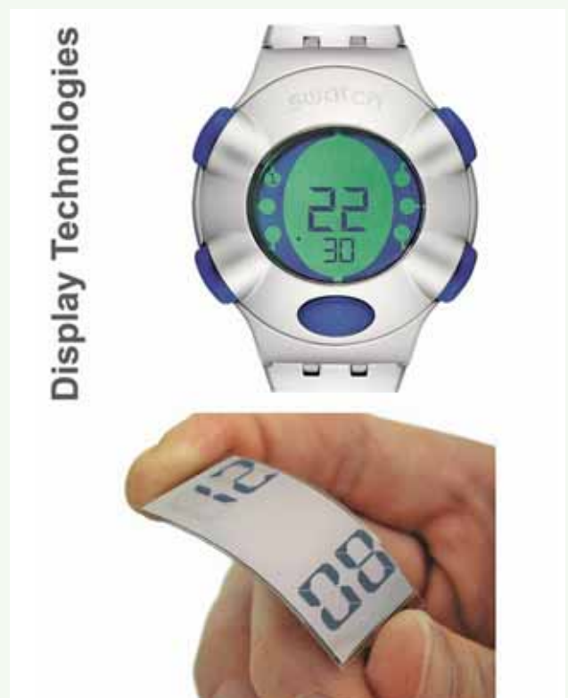
Fig. 4: From multifunctional watch (Swatch Beat) to flexible plastic LCD displays
