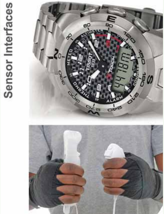
Fig. 8: Sensor interfaces in Tissot T-Touch and game controller with 3D acceleration sensors
