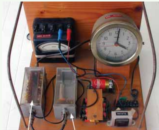
10 kHz quartz oscillator 4 divide-by-ten stages
