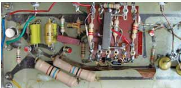
Fig. 7: Experimental phaselock loop frequency divider. It includes a 8kHz oscillator based on an early quartz prototype.
