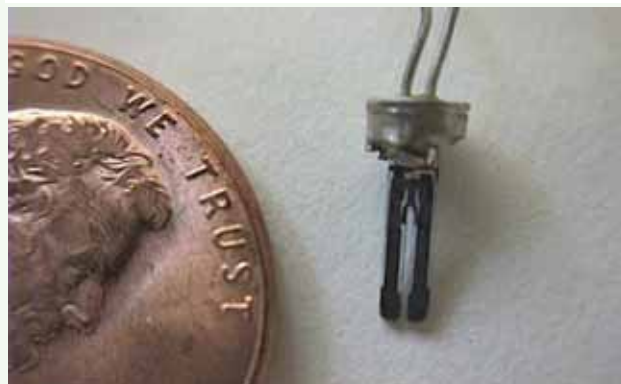
Figure 8 – Quartz tuning fork resonator of Juergen Staudte [26][27]; typical unit shown on bottom with cover removed (photo credit: Erhard Schreck)
